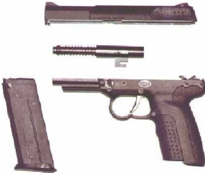
Five-sevenN Tactical (note safety switch above the trigger)
